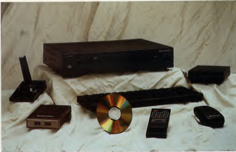
The complete CDTV set up with its infra-red remote control joystick and mouse. What you are looking at is basically an Amiga with a CD-Rom drive attached. It looks slick in a black box though.
